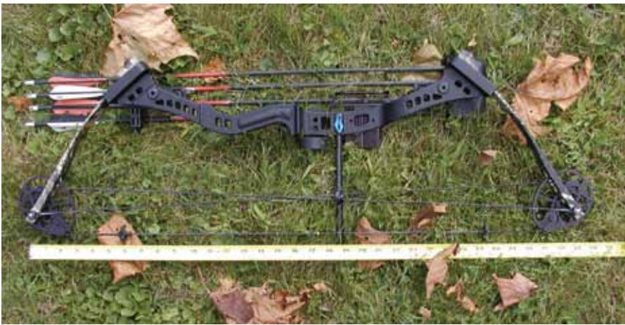
My friend Tony bought this Diamond youth for his growing daughter, Makenna. The cams are small on this 33 inch axle-to-axle bow to control the draw length. The bow draws to a moderate amount of peak weight and holds it there through the remainder of the draw stroke allowing the youth to draw to their proper full draw position whatever it is.
